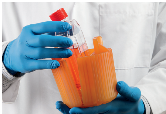
Figure 3. Flasks are easily inserted into the adapter. With adapters for the Corning 75 cm 2 canted-neck flasks, insert with thick-seam side facing the direction of the arrows on the adapter top; or insert the canted-top tilted toward the side of the adapter with the arrows. Adapters for Corning 25 cm 2 canted-neck flasks can tilt in either direction.
