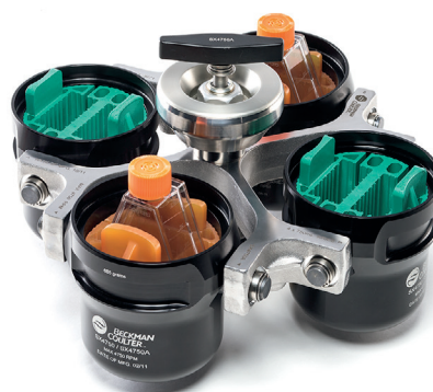
Figure 4. Easily load the adapter into the bucket by grasping the adapter finger grips. Align the narrow sides of the flask to the bucket engraving and the wide sides parallel to the bucket pin pockets.
